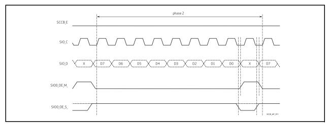
Figure 3-9 Phase 2 — Sub-address (3-Phase Write Transmission)
