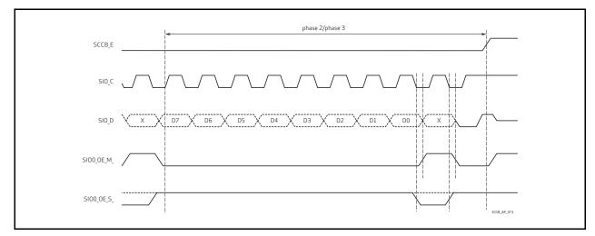
Figure 3-11 Phase 2 Sub-address Write Transmission/Phase 3 Write Data Transmission
